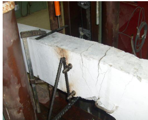
Figure (7) Failure of Control Column
