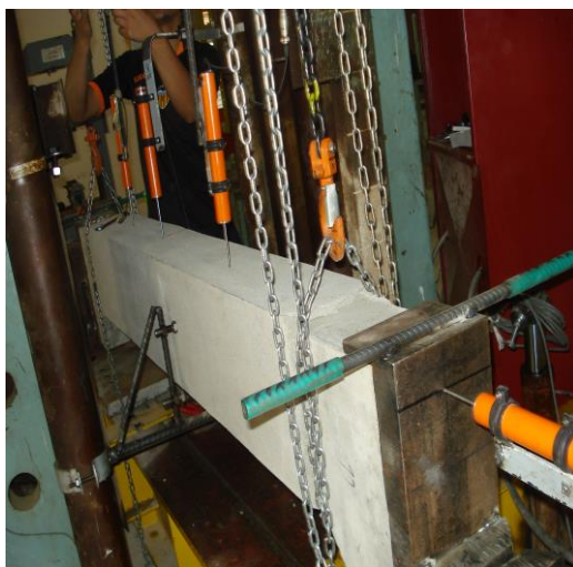
Figure (4) Experiment Set up Showing Position of Transducers.
